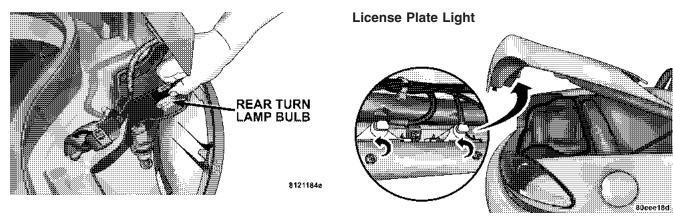
Twist off sockets counter-clockwise and pull out bulbs. Replace as required.
